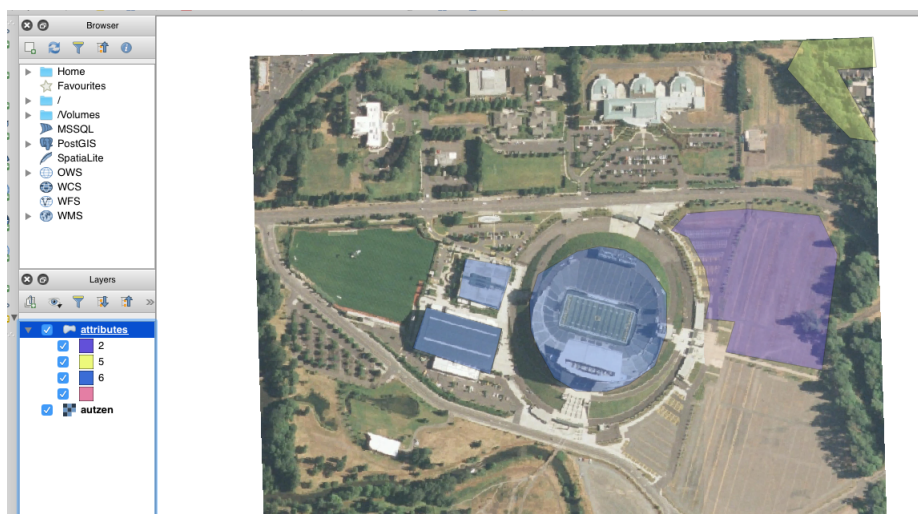
Fig. 12.11: We want to clip out the polygon in the upper right hand corner. We can view the GeoJSON ( http://geojson.org ) geometry using something like QGIS ( http://qgis.org )
